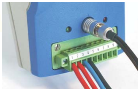
Input channels and serial PC interface port
